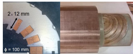
Fig. 9. Left: Collar with slots filled with Nb-Ti conductors. Right: Half of a 4.4 T dipole made of the motor-like collar technology [21].
