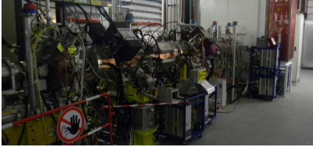
Figure 2: The 3 MeV injector in the Linac4 tunnel. From the right, ion source, RFQ, chopper line.
