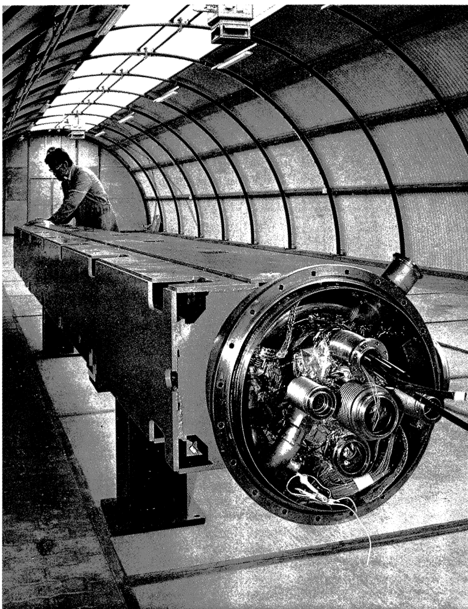
Six-metre superconducting bending magnet for the proposed HERA electron-proton machine ready for tests at DESY.
