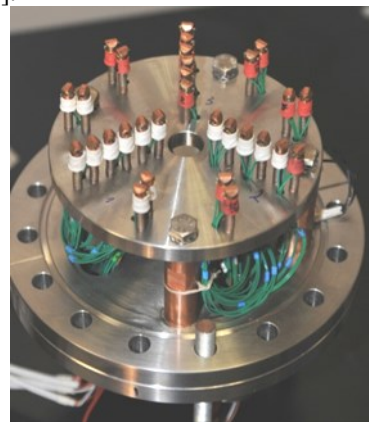
Figure 6: repartition of thermal sensors and the calibrated heater on the backside of the sample.
