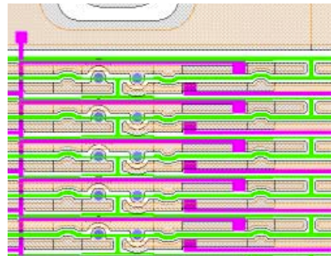
Figure 12: Detail of the poly-silicon biasing scheme for a sensor with 25 \times 500 \mu\text{m} pixels designed by the ATLAS Japan Silicon group and produced by Hamamatsu Photonics KK. The biasing lines are staggered on neighboring pixels.
