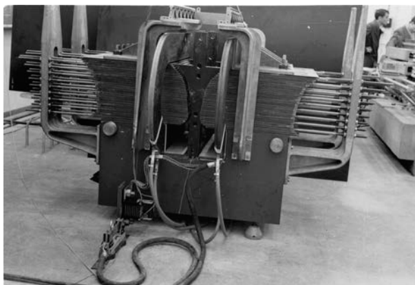
Fig. 1. The adjustable pole model for PS magnet development.
