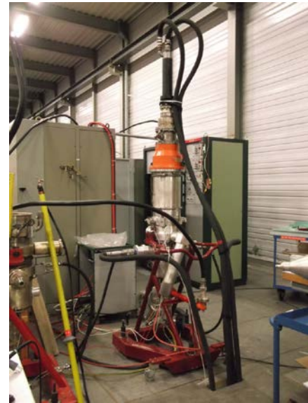
Figure 10 Cryomodule and RF system layout in the BA4 cavern (left) and a 400 MHz Tetrode amplifier under test (right).
