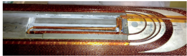
Figure 9: Correction to the loop adopted in MQXC2.
