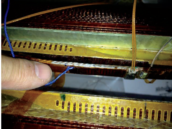
Figure 4: A view of the quench heaters with their cooling slots mounted between layers. We also see the spot heater and adjacent voltage taps.
