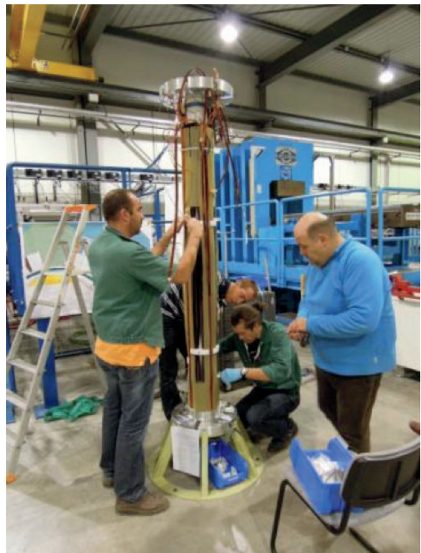
Figure 1: Vertical assembly of the coils around the collapsible mandrel, and open ground insulation around the coils.
