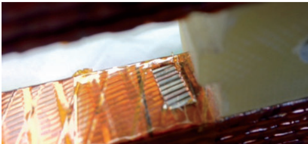
Figure 4: A view of the quench heaters with their cooling slots mounted between layers. We also see the spot heater and adjacent voltage taps.
