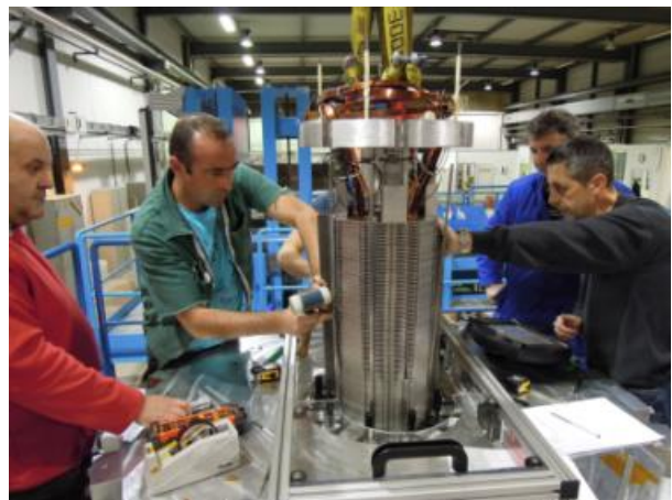
Figure 3: A view of the final stage of collaring.
