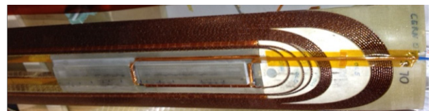
Figure 8: Inductive loop formed by the voltage taps coming from the interlayer joint in MQXC1.
