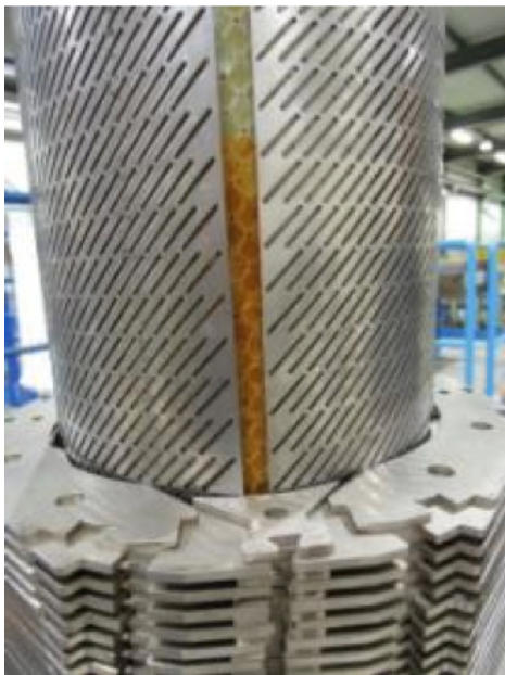
Figure 2: Assembly of the collared coil: view of collars before compression, and collaring shoes with openings.
