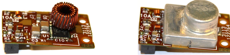
Figure 4. Photographs of a PIX_V10 DC-DC converter, without (left) and with (right) the shield attached.
