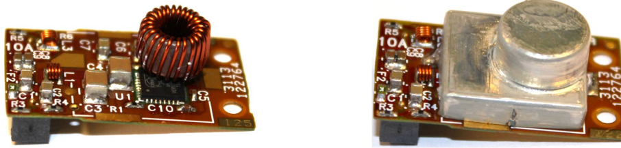
Figure 4. Photographs of a PIX_V10 DC-DC converter, without (left) and with (right) the shield attached.
