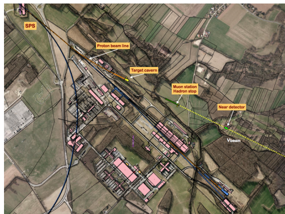
Figure 2: The baseline layout for the CN2PY neutrino facility in the vicinity of the SPS North Area.
