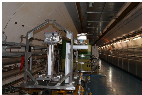
Figure 5: The HRMT10 setup with the side mounted mirror used for the fast photography and laser vibrometry from a 40 m distance where the camera and laser control box are located.
