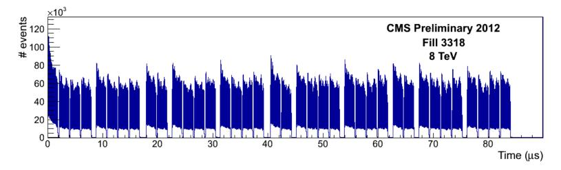
"Cumulative full-orbit histogram from the Real-time Histogramming Unit (RHU) used by the fast beam condition monitor BCM1F. Hits from a single BCM1F sensor are histogrammed in 14256 bins per orbit (4 bins per bunch crossing) for a proton-proton fill. The spacing between bunches is 50 ns. The structure of the bunch trains is clearly visible within the orbit."
