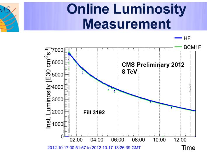
"Instantaneous luminosity measured by the fast beam condition monitor BCM1F and the forward hadronic calorimeter HF, plotted as a function of time during a single fill. The BCM1F value was normalized to HF at a previous point in time. This plot shows how well BCM1F tracks HF within that normalization, showing BCM1F's suitability to complement HF as an online luminometer."
