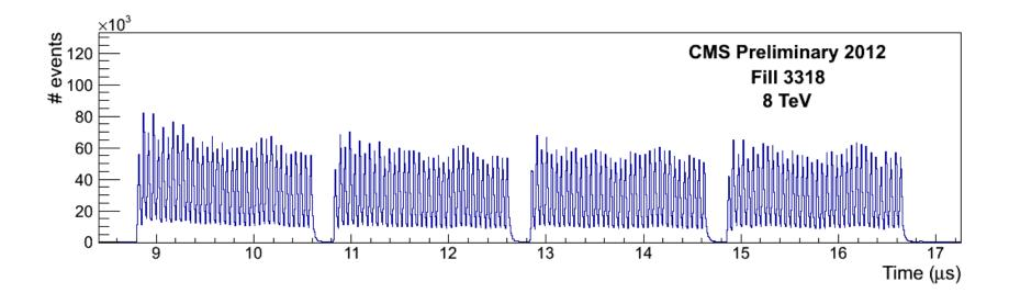
"Zoom-in of cumulative full-orbit histogram from the Real-time Histogramming Unit (RHU) used by the fast beam condition monitor BCM1F. Hits from a single BCM1F sensor are histogrammed in 14256 bins per orbit (4 bins per bunch crossing) for a proton-proton fill. The spacing between bunches is 50 ns. The structure of the bunches is clearly visible within the bunch trains."
