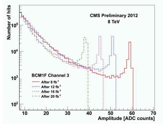
"A single BCM1F channel's amplitude spectrum (in ADC counts) plotted for several values of integrated luminosity. The endpoints indicate the saturation amplitude of the front-end 1310 nm laser driver and take into account the baseline subtraction algorithm. The saturation amplitude decreases with integrated luminosity, showing successive radiation damage of the laser driver. BCM1F receives approximately 2.9e12 cm<sup>-2</sup> hadron fluence per fb<sup>-1</sup>."
