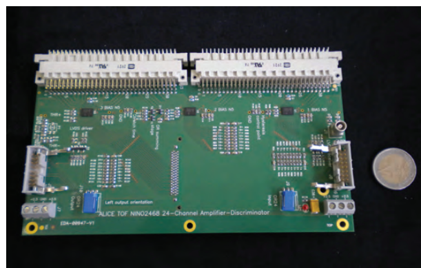
Fig. 5. The 24-channel NINO card designed for the ALICE experiment and used in our tests.
