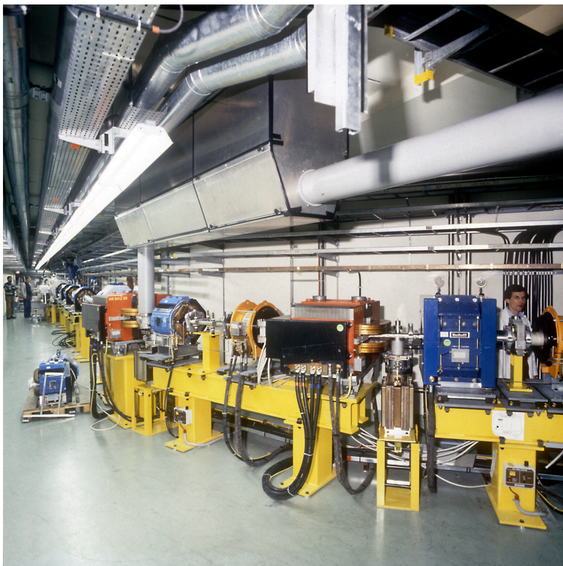
Fig. 2: Arc and straight section of the EPA. Red: bending magnets; blue: quadrupoles; yellow: sextupoles. The white vertical and horizontal tubes above the arc guided the light to the synchrotron radiation monitor.
