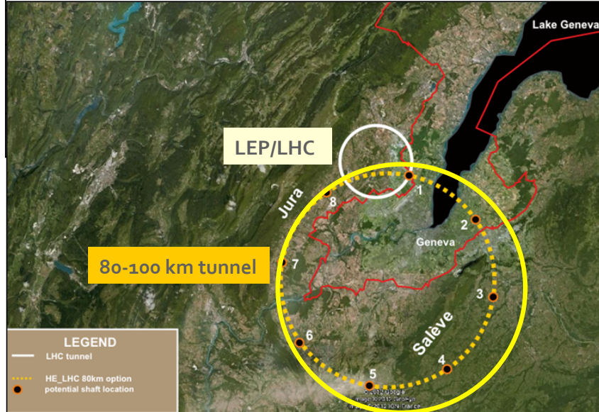
Fig. 2: A possible implementation of the 80 km tunnel (dashed circle) that would host TLEP and the VHE-LHC in the Geneva area, taken from Ref. [9]. The 100 km version (full line) is currently under study.
