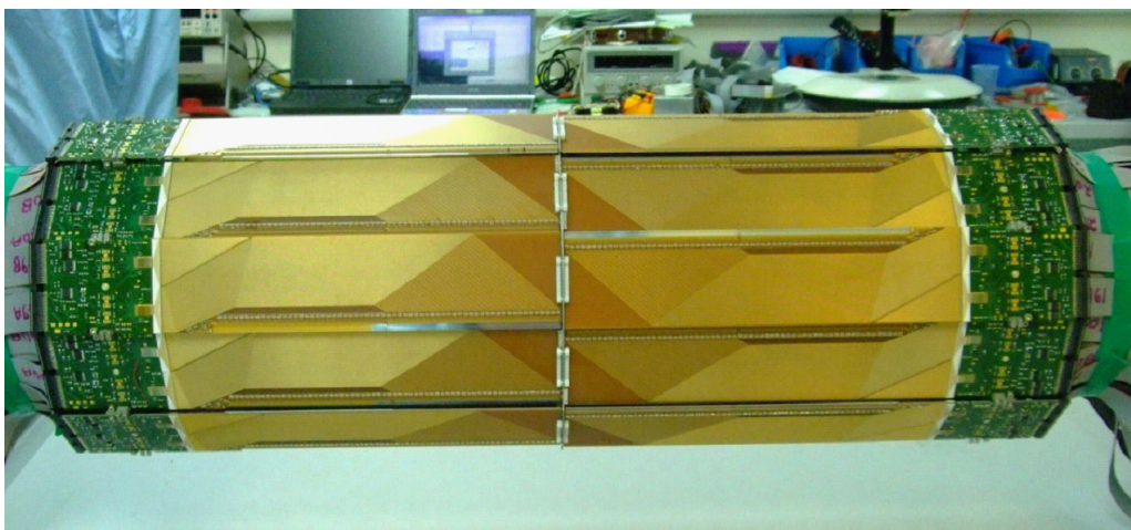
Figure 2. Detector in its mount frame before sealing the outer covers.
