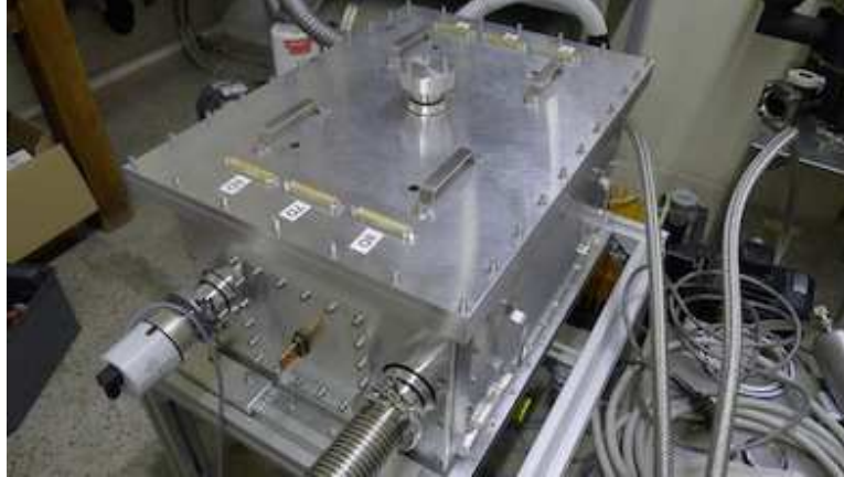
Figure 2. Photo of the VIP2 box assembled for first tests in the laboratory.
