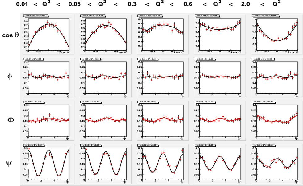
Fig. 3. The distributions  $\mathcal{W}(\cos\theta)$ ,  $\mathcal{W}(\phi)$ ,  $\mathcal{W}(\Phi)$  and  $\mathcal{W}(\psi)$  in 5 bins of  $Q^2$  (shown at the top of the figure). Experimental results are shown with dots, vertical bars represent the statistical errors alone, longitudinal bars show angular bins. Solid curves are results of the fits discussed in a text.
