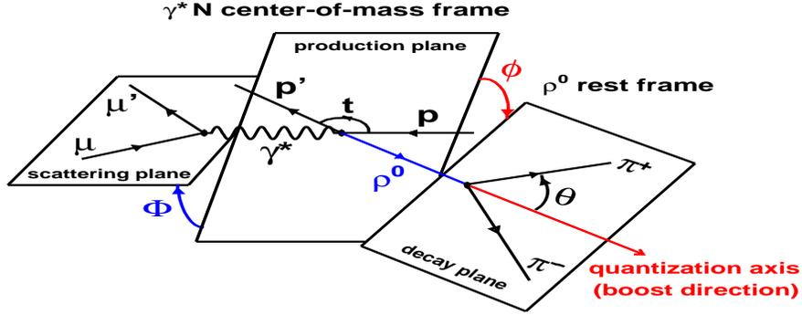
Fig. 1. Angles and planes used to describe exclusive  $\rho^0$  production and decay.
