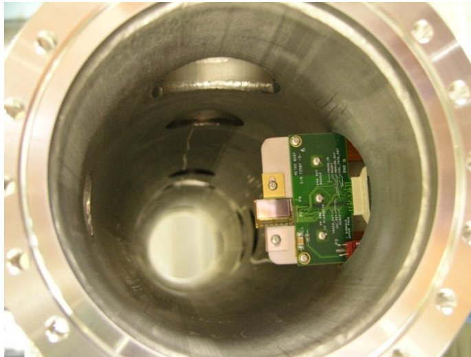
Fig. 5. This image is of a single pixel assembly within the vacuum chamber. The view is from upstream towards downstream through the center of the vacuum vessel.
