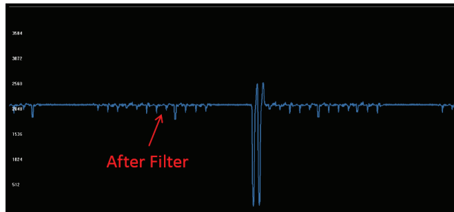
Fig. 8. This figure shows the analog output from one plaquette after the software-based filter approach was applied. It can be seen that the spikes were reduced substantially when compared to Fig. 7.
