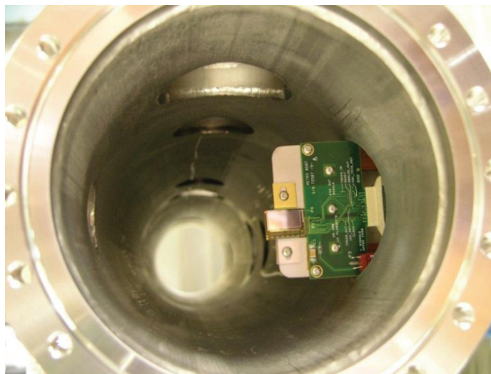
Fig. 5. This image is of a single pixel assembly within the vacuum chamber. The view is from upstream towards downstream through the center of the vacuum vessel.
