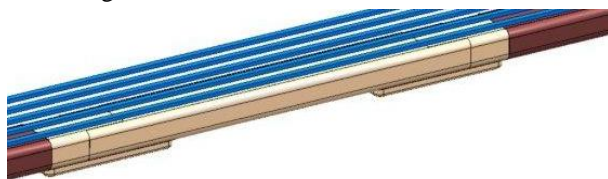
Figure 2: Design of the consolidated quadrupole magnets bus splice showing two electrical shunts and spool pieces bus bars.
