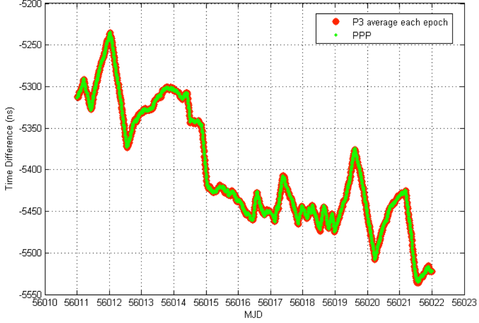
Figure 6. CERN and LNGS clocks time differences as estimated with P3 and PPP algorithms for the period MJD 56011-56021, corresponding to 2012 March 25 th - April 4 th .
