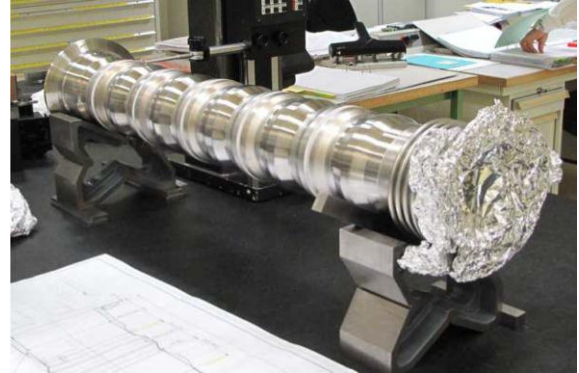
Figure 11: 5 gaps vacuum chamber.
