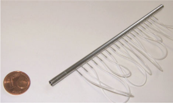
Fig. 39. Prototype of a gas distributor consisting of a stainless-steel pipe (4 mm diameter, 0.1 mm wall thickness) with small capillaries (0.55 mm diameter) for connecting the individual straws.
