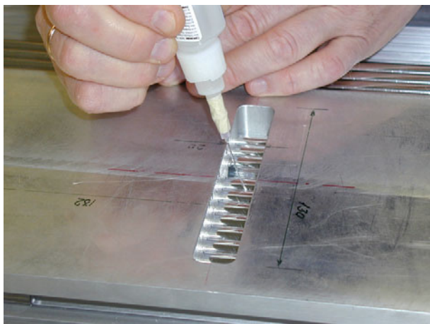
Fig. 26. Gluing of straw tubes to multi-layers.
