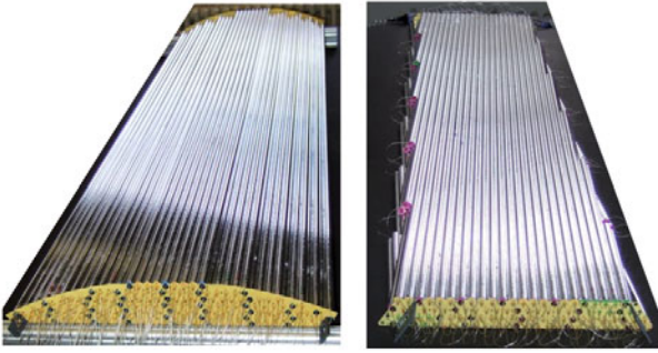
Fig. 24. Photograph of an axial straw layer module for the outer cylindrical shape and module with two double layers with opposite skew angle.
