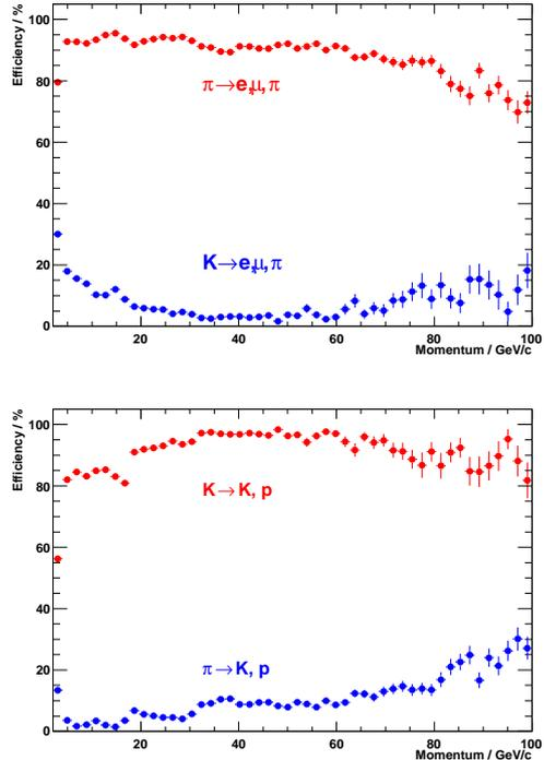
Fig. 9. The efficiencies and misidentification probabilities (in %) as a function of momentum for pions identified as “light” (top) and kaons identified as “heavy” (bottom).
