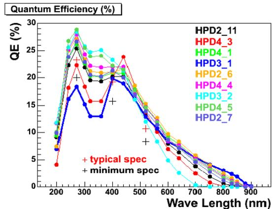
Fig. 5. The measured quantum efficiencies of nine pre-series HPDs.
