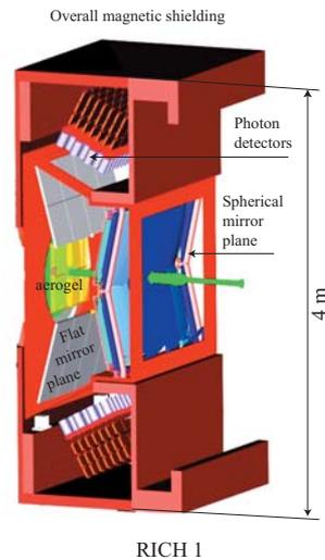
Fig. 2. A schematic of the RICH 1 detector.
