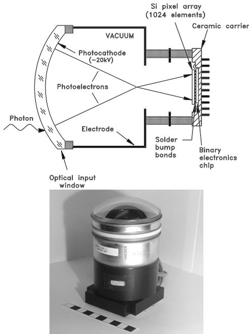
Fig. 4. Schematic of a Hybrid Photon Detector and photograph with a 10 cm scale.
