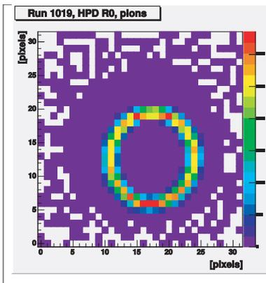
Fig. 6. Ring image on an HPD from a 10 GeV/c pion beam and  $\text{N}_2$  radiator, integrated over  $\sim 30\text{k}$  events.
