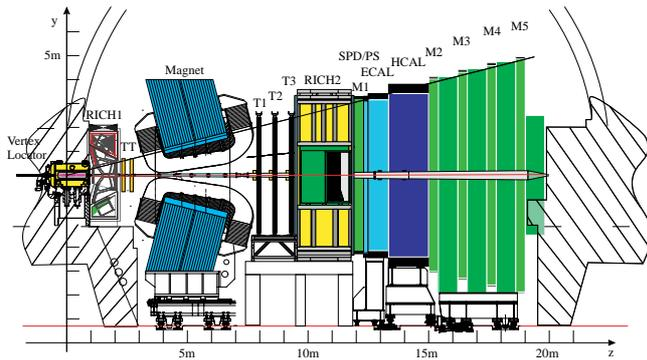
Fig. 1. A schematic of the LHCb detector.
