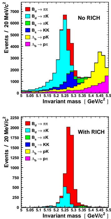
Fig. 10. The effect of the RICH in the selection of the channel  $B \rightarrow \pi^+\pi^-$  without (top) and with (bottom) using RICH information.
