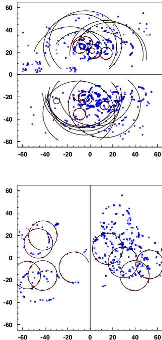
Fig. 8. Distributions of hit HPD pixels on the HPD planes of RICH 1 (top) and RICH 2 (bottom). Units are in cm.
