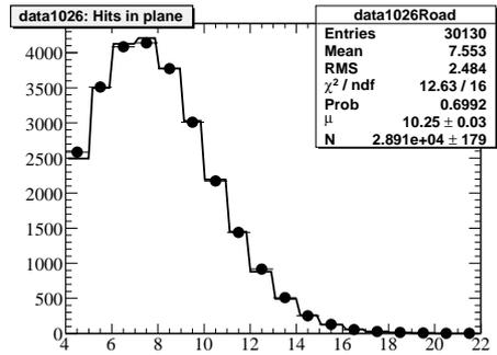
Fig. 7. The number of PEs observed on a single HPD (points). The Poisson fit to these data is also shown (solid line).
