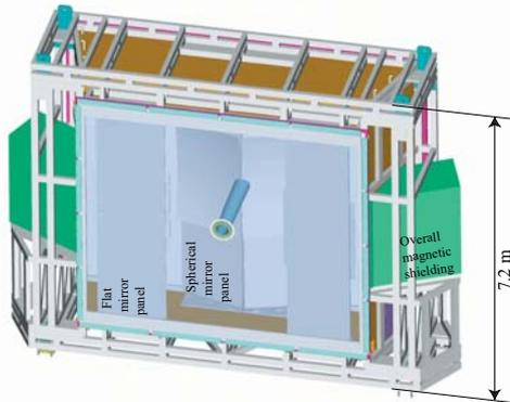
Fig. 3. A schematic of the RICH 2 detector.
