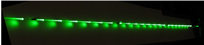
Fig. 15. View of the optical fiber with notches. The fiber is illuminated by a continuous light to visualize the notches.
