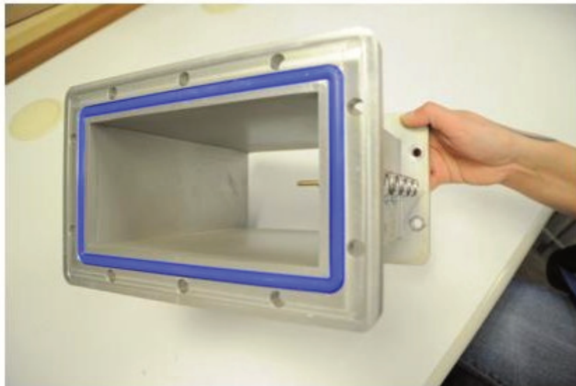
Fig. 7: Waveguide with damping antennas on the small side of the waveguide
