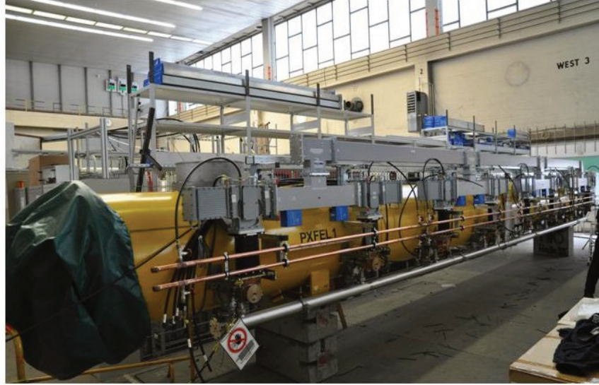
Fig. 5: Accelerator module and RF waveguide distribution
