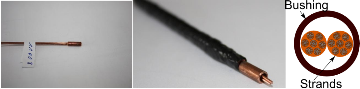
Figure 2: Photograph and cross-section of Nb_3Sn strands connected to a Cu-bush with EMPT.
