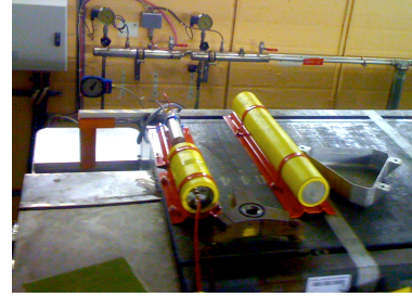
Figure 3: Test BLMs installed on top of the main magnet. The detectors are installed according to Fig. 2
