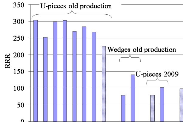
Fig. 4. RRR of different Cu profiles used for the assembly of the LHC main busbar interconnection splices.
