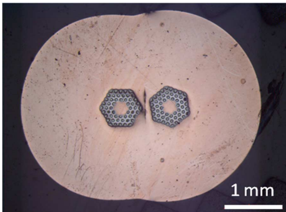
Fig. 2. Metallographic cross section of an unreacted \text{Nb}_3\text{Sn}/\text{Cu} lap joint produced by electrolytic deposition of a 1.2-mm-thick Cu layer on top of two \text{Nb}_3\text{Sn}/\text{Cu} RRP strands ( \varnothing = 0.8 mm).
