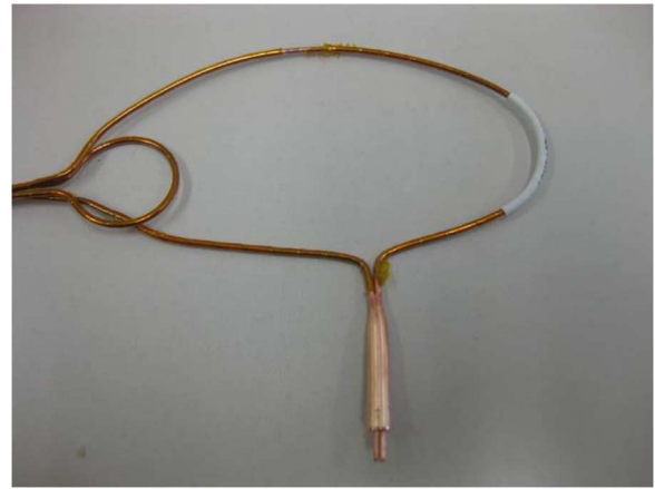
Fig. 3. Nb-Ti/Cu test loop for the measurement of the joint resistance. The joint has been produced by electrolytic Cu deposition.
