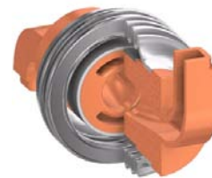
Figure 10: 3D model of the double-sector choke flange.
