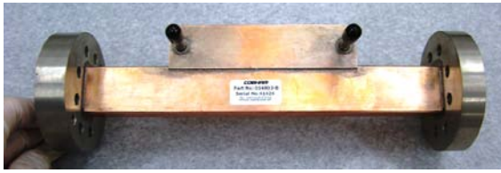
Figure 5: Bi-directional coupler by Cobham Microwave
