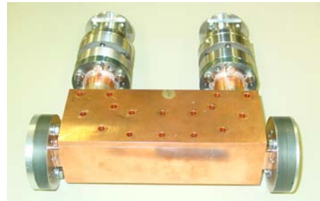
Figure 3: Bi-directional coupler by GYCOM Ltd
