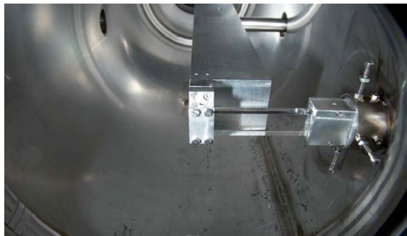
Figure 7. Tungsten absorber at TACW.51998 with quartz Cherenkov radiator. The radiator is clamped to the tungsten bar to the left and can slide through the left support whilst the absorber is moving. The sliding box ends with a window through which the Cherenkov light can be collected.
