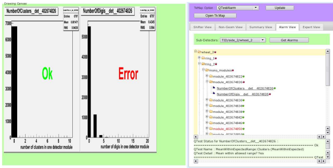
Fig. 4. The alarm view panel showing the alarm tree for a specific layer of SST. In the drawing canvas two histograms are shown where one of them passed the QTest but the other one failed. The result of the rest is displayed in the message window .
