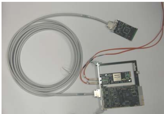
Figure 3. Picture of the S-link64 CMC (top-right), LVDS cable, FRL with Myrinet NIC.
