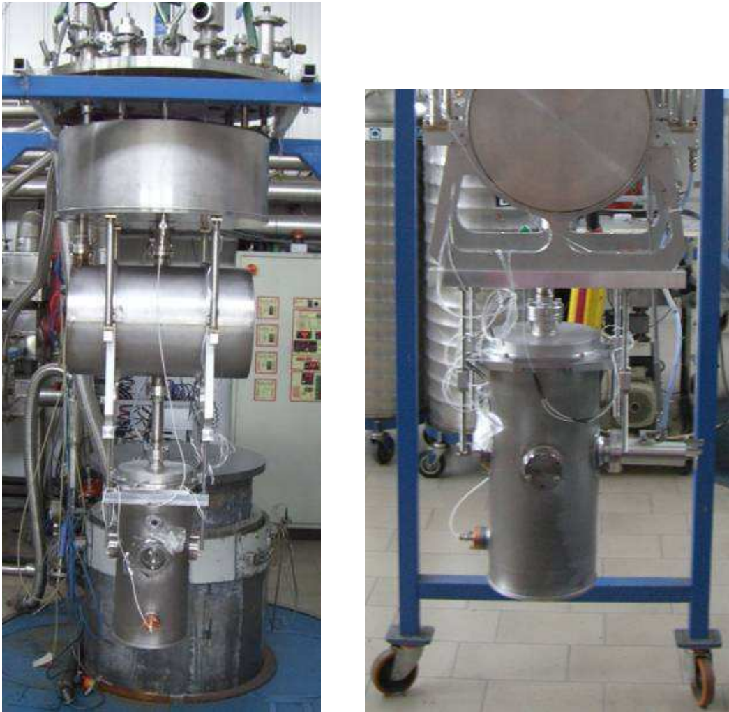
Fig. 4 : Half-wave resonator mounted on the cryostat insert just before the cold test
