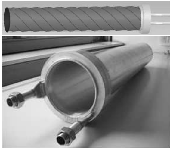
Fig. 2. Upper panel: design sketch of the inner part of the double-walled cryopanel showing the spiral structure separating the six gas flow channels. Bottom panel: photograph of the cryopanel prototype.
