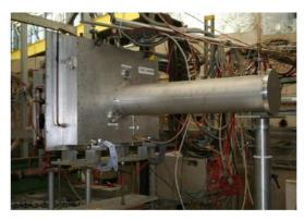
Fig. 5. The radiator of the prototype detector. The mirror is located at the end of the tube.
