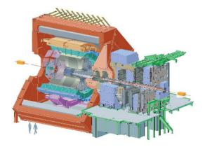
**Fig. 1.** The schematic view of the present ALICE experiment. The VHMPID is likely to take place in the bottom part, around the PHOS detector (shown in purple).
