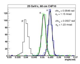
Fig. 4. Simulated Cherenkov angles for different particles
