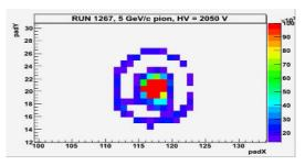
**Fig. 6.** 5 GeV/c pion beam crossing the prototype during the beam-test [13]. Place of the incident particle is visible in the middle while the Cherenkov ring is located around it.
