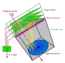
Fig. 2. Operation of the VHMPID detector
