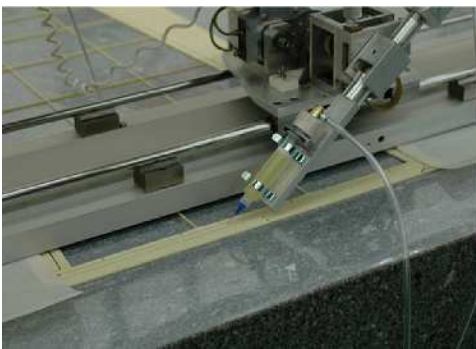
Fig. 6. GE1/1 Gluing spacers on the foil with the glue gun.
