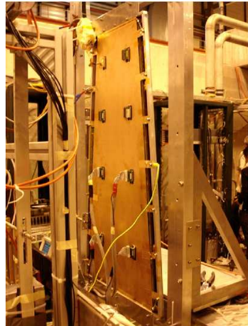
Fig. 11. GE1/1 Installed at the Test Beam.
