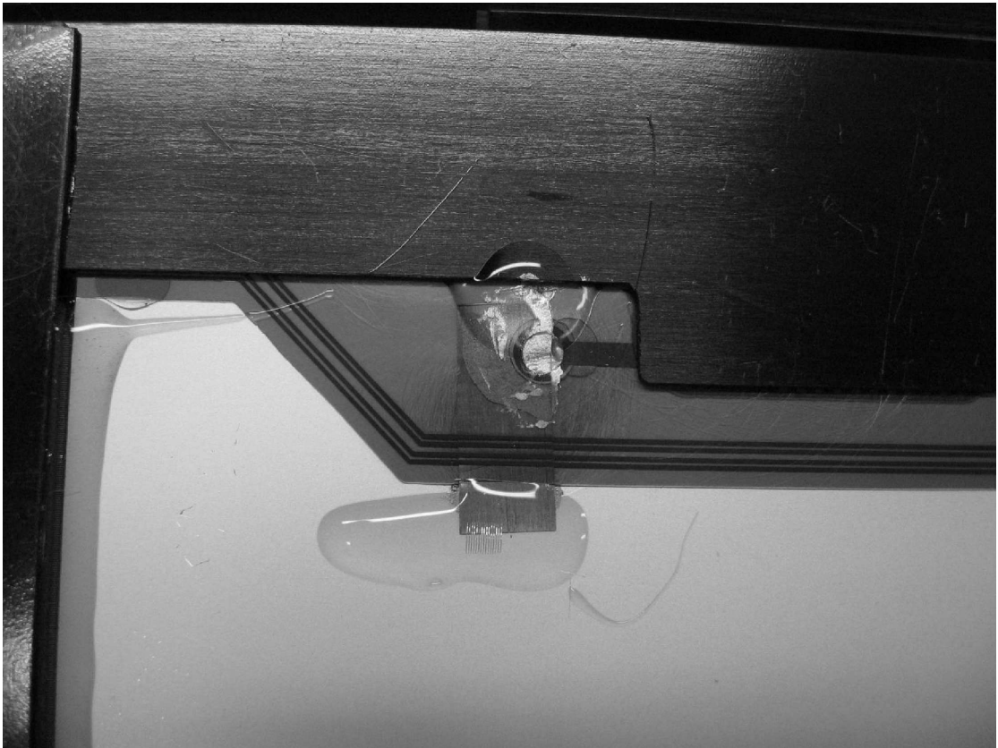
Figure 6.22: Photograph shows silver epoxy deposited imprecisely, which resulted in an electrical short between the bias line and the module carbon-fiber frame.
