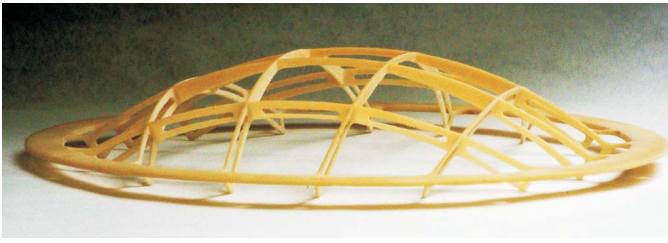
Figure 7. A curved spacer made by stereolithography.
