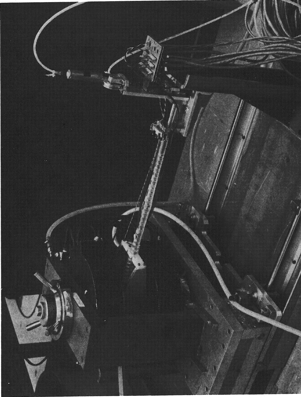
Fig. 6 Apparatus used to calibrate the flip-coils. The electromagnet at the left of the photograph is mounted on ways and can be positioned over any of the 40 flip-coils or an NMR probe just beyond the end of the flip-coil arm (the position shown in the photograph). The pneumatic cylinder and pulley arrangement used to flip the coils is seen at the right.
