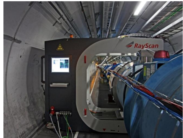
Figure 4: The RayScan Mobile X-ray Tomograph in operation at the LHC.
