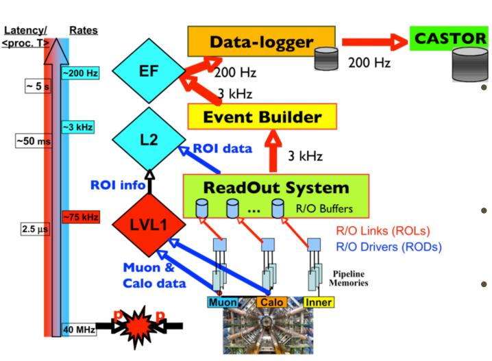
Three-level trigger architecture to achieve a final rate of 200Hz, from the 40MHz collision rate
