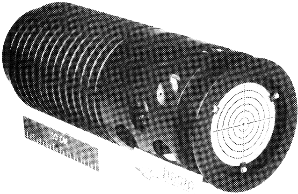
Fig. 5 - Overall view of the target assembly. The aluminium container is anodised black to aid cooling via radiation. The hole in the upstream luminescent screen avoids premature aging and radiation damage of the latter.
