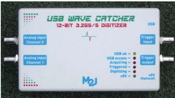
Figure 4: the USB Wave Catcher box
