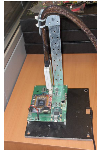
Figure 4: Former Test Board for VFE
