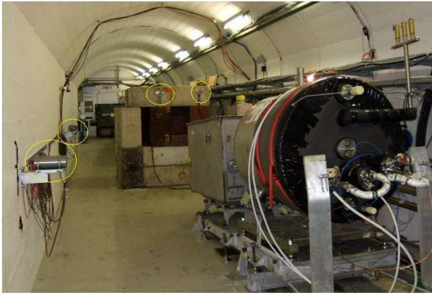
Figure 2: The experimental setup in the TT2A tunnel. The yellow circles indicate the location of four of the six detectors: the two in the forward direction are at 10 deg. angle from the target, and the other two at 20 and 90 degrees respectively. A fifth detector is located behind the beam attenuator and the sixth at 20 deg. on the beam-right behind the experimental setup.
